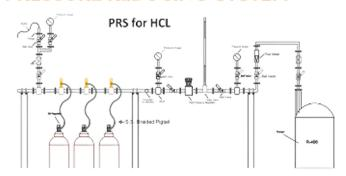
PCI make Pressure Regulation System is the most safest method of using flammable & corrosive gases as it has built-in safety shut off arrangement with 100% redundant safety measures. Additional safety interlocks can be incorporated as per process requirements. Provision of Nitrogen purging for safe operation.
